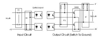
The circuit diagram of inputs and outputs is shown in figure 2. Inputs have common ground. The outputs either switch to ground or to supply voltage.
