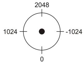
**2. Zero point adjustment without sign:** Parameter 0-04 have to be programmed to 0
